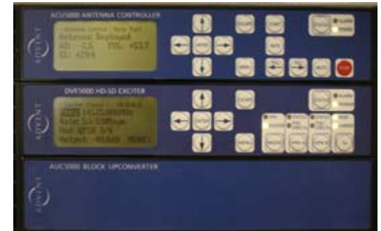
ACU5000, DVE5000 and AUC5000 showing front panel display
