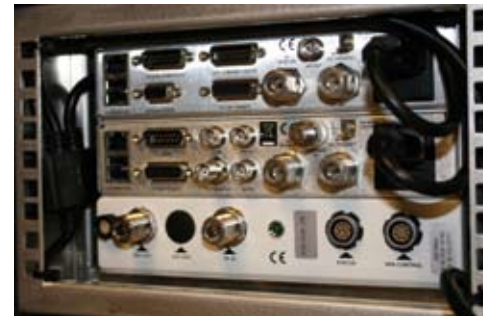
Half rack flight case, housing three 5000 series units. Flightcases are available in variety of options to suit the application
