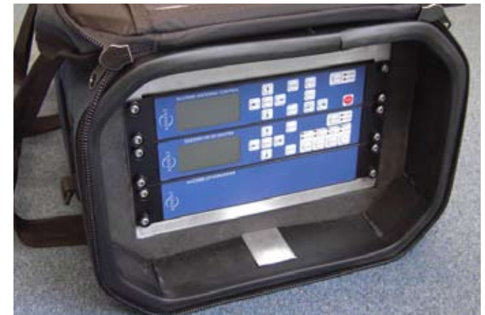
Half rack flight case, housing three 5000 series units. Flightcases are available in variety of options to suit the application
